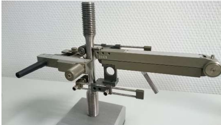
Pic. 2: Illustrative photo of two extensometers on a cylindrical sample with threaded heads.
