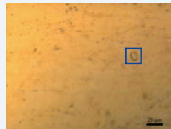
Observation Image of Contaminant on Terminal Magnified by 15x with Cassegrain Mirror
